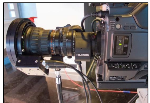
Figure 12 Remotely operated filter rotator
